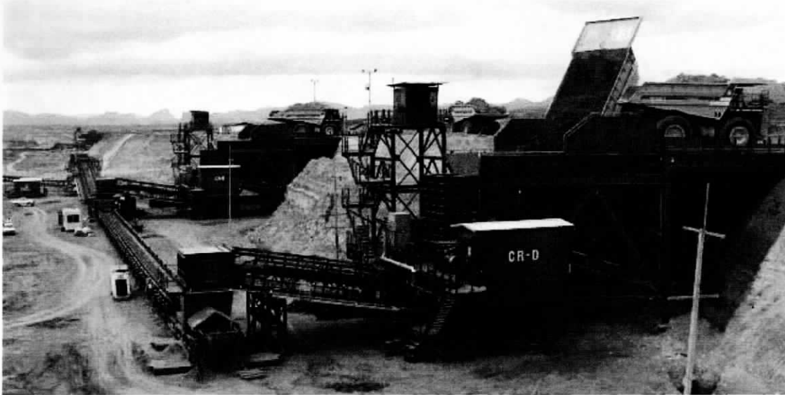
Figure 2. Semi-mobile crushers feeding one overland conveyor
