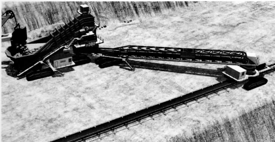
Figure 3. PF300 fully mobile crushing system consisting of a loading shovel, the mobile crusher, a belt bridge and a track-shiftable bench conveyor
